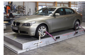
Special pallet for transport of cars
