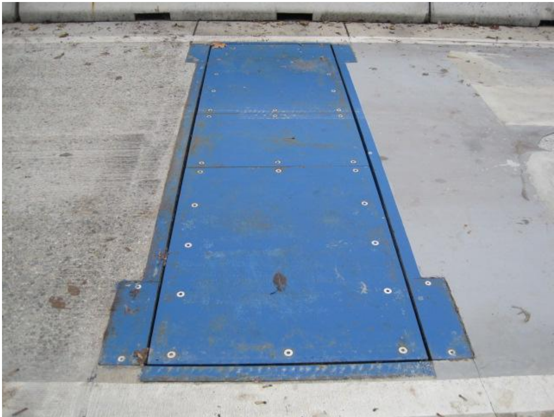
Figure 9 Each axle of the vehicle is weighed, one at a time, by driving of the vehicle slowly over the scale.
