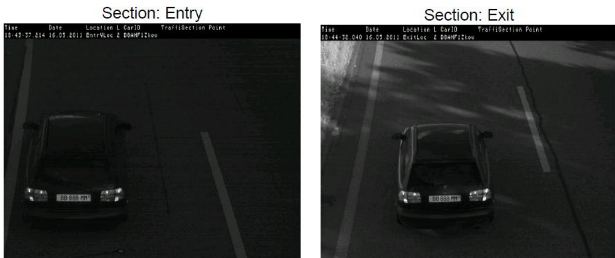
Figure 2 The vehicle's registration plate is scanned at the beginning and end of the measurement, after which the vehicle is photographed from the front to identify the driver and for comparison of the registration plate to the image scanned from the rear.
