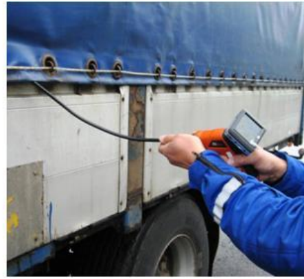
Figure 13 On the left, the video endoscope is used to inspect narrow spaces in a vehicle's structures; on the right, how to inspect the load without opening the covers.
