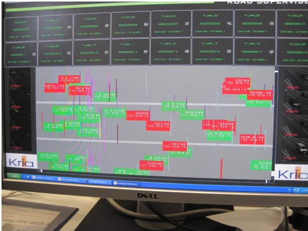
Figure 5 A separate speed measurement system using KRIA 3D speed cameras was installed on the motorway before the checkpoint to measure the speeds of passing vehicles via video technology
