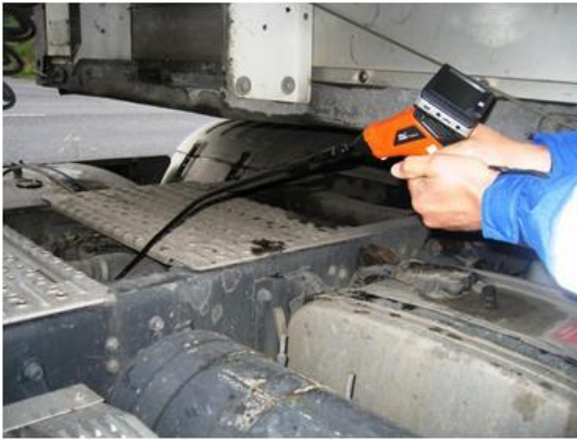
Figure 13 On the left, the video endoscope is used to inspect narrow spaces in a vehicle's structures; on the right, how to inspect the load without opening the covers.
