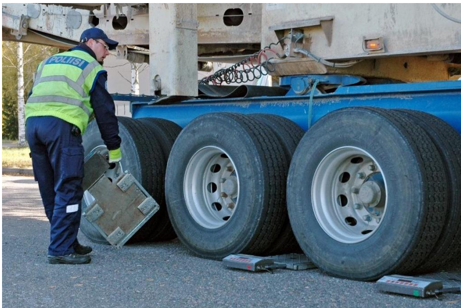
Figure 6 Weight control of HGV with one scale per axle
