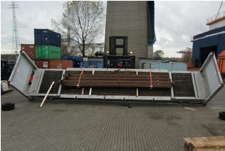
Figure 8 Tilting of a container to test the securing of freight
