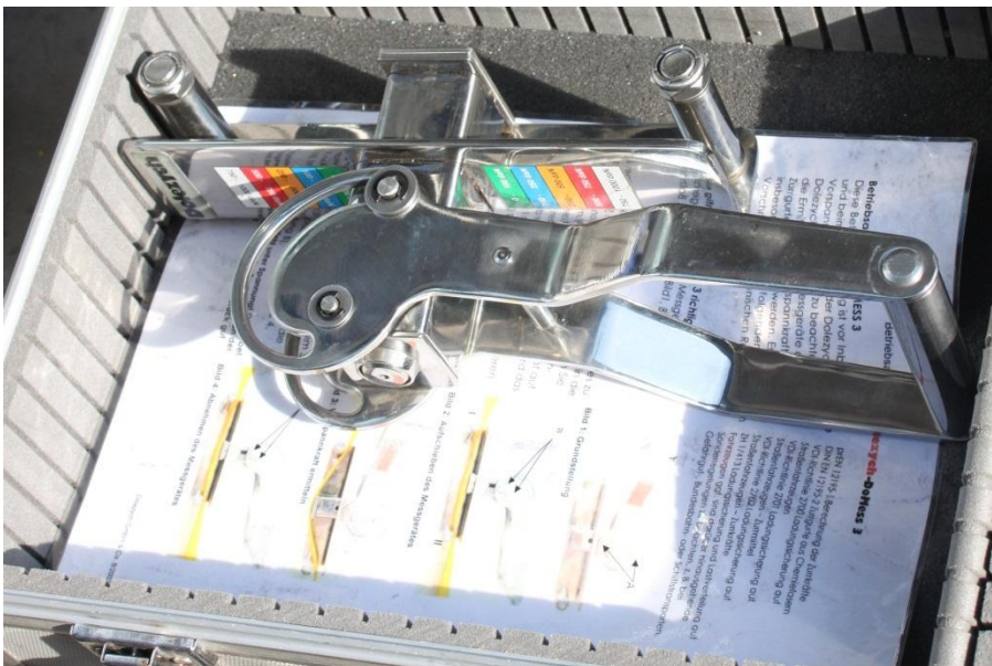
Figure 9 Instrument to test the tension of cargo straps
