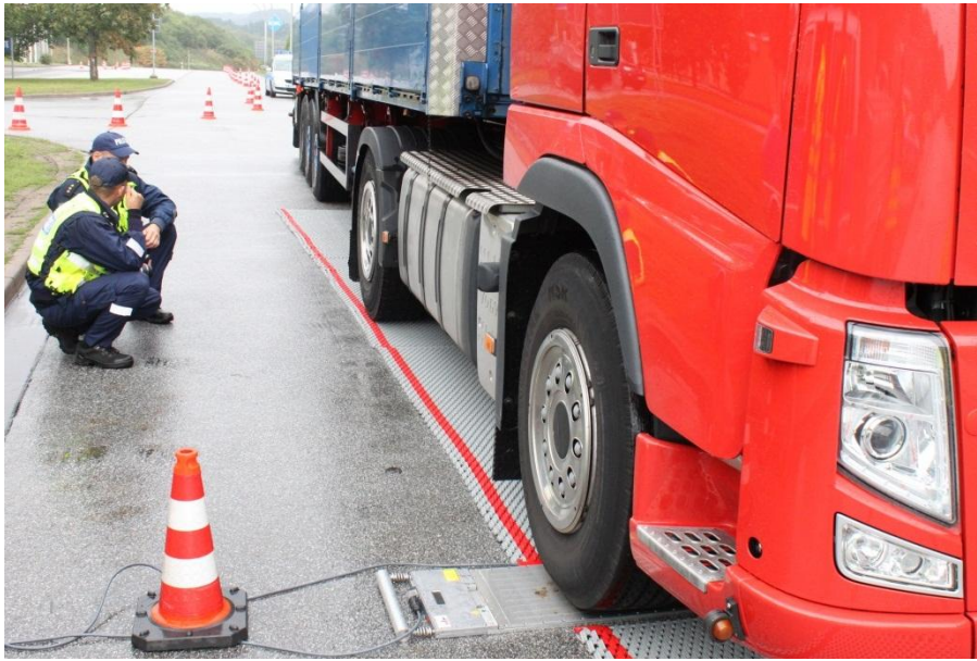
Figure 5 Weight control of HGV with 2 scales and levelling mats
