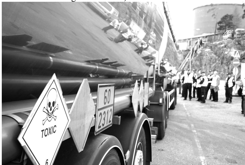
Figure 1 Example of appropriate labeling of tank truck (Photo: Author)
