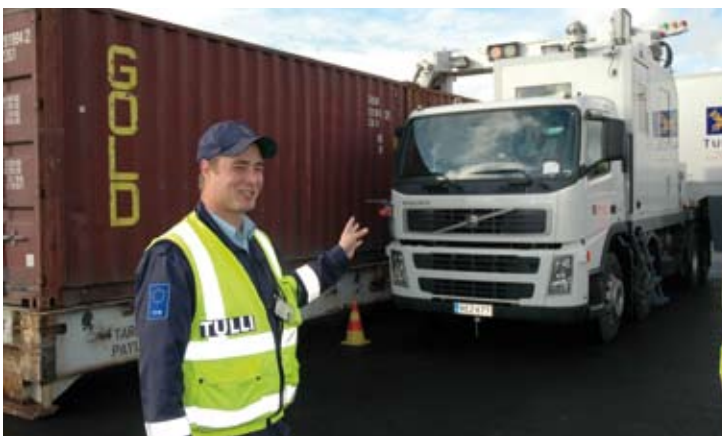
Mobile X-Ray installation of the Finnish Customs for inspection of containers, Photo: TuTech
