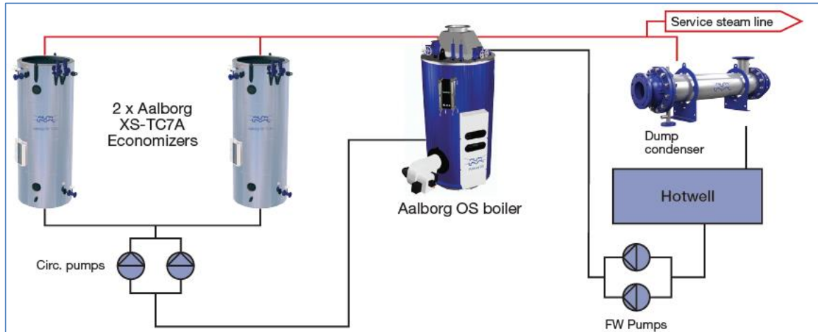
Figure 3. 10: Simplified layout of case ship's auxiliary WHR subsystem
