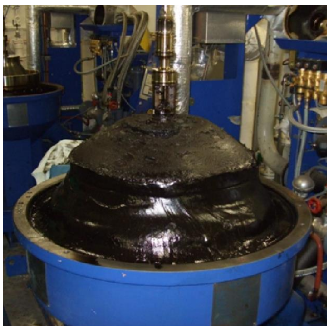
Figure 7. 4: Fully contaminated and blocked fuel centrifuge [9]
