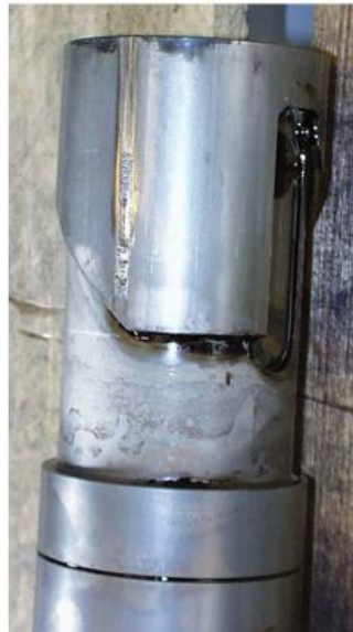
Figure 7. 5: Damaged plunger of the injection pump as a result of too rapid change of the residual fuel to distillate, low sulphur fuel
