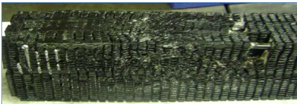
Figure 7. 3: Defective electric fuel heater
