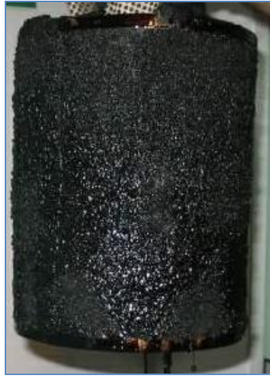
Figure 7. 1: Heavily stained and blocked fuel filter of the transfer pump
